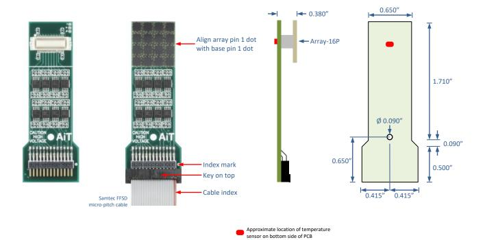
Measurement tolerance: ±0.020"
